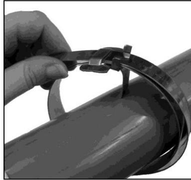
2. Insert band around workpiece again and through buckle. *Double wrapping develops much more radial compression than single wrapping.* Bend end of band under buckle.
