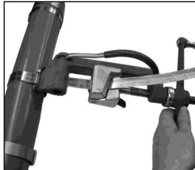
5. *Roll tool over buckle, backing off with Tension Handle 1 - 1½ turns throughout entire rolling operation.* Failure to back off tension with tension handle throughout roll-over may result in breaking the band. There is no loss of tension as band released is used up in this process.
