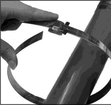
1. Slide buckle on band as shown. Bring tip of band around workpiece and again through buckle.
