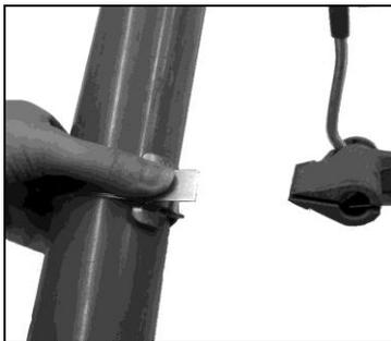
7. Remove tool, holding stub of band down.
