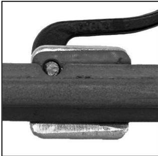
1. To remove Gripper, align Gripper Pin hole with notch in tool frame. Using a punch and hammer, punch Pin out of Slide Block.
