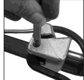
3. To replace Pin, Gripper Spring must be seated in Tension Screw hole. Align Gripper hole with Slide Block hole and insert Pin using a hammer.
