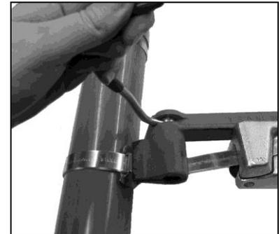
6. Rotate Cutting Handle forward to cut the band. When applying Giant Band clamps, prior to cutting off clamp, release Band Gripper and push Tool Nose away from buckle approx. ¼".
