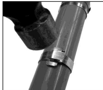
8. Hammer down buckle ears to complete BAND-IT clamp.
